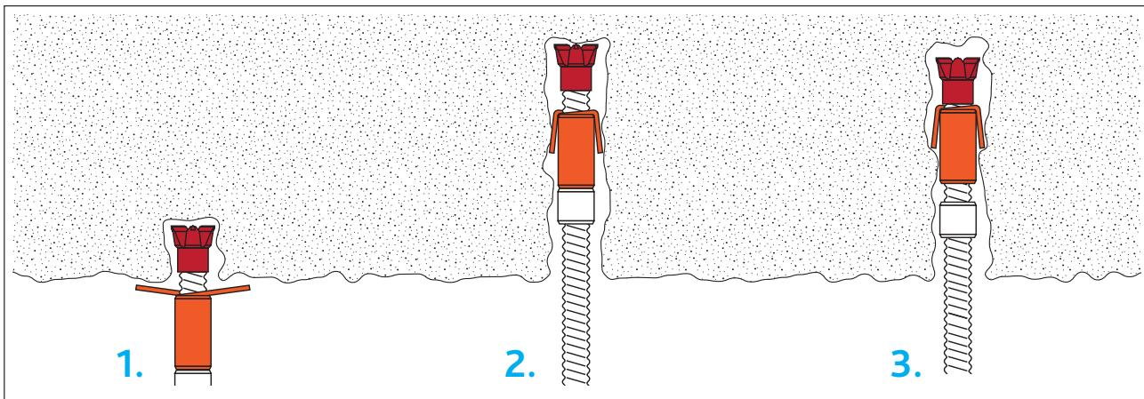
The *SDA LOCK* abuts the shoulder during drilling, the *SDA* rotates independently within the *SDA LOCK*. **1 & 2**
