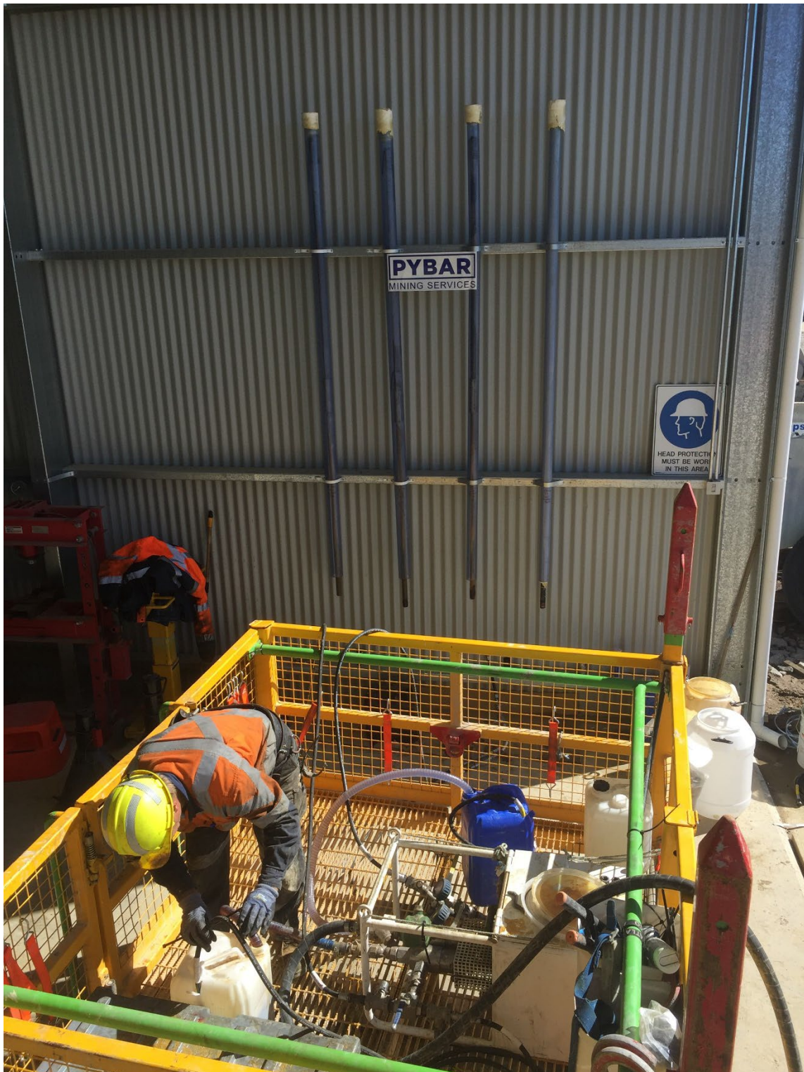
FIG 6 – Resin encapsulation tests using Perspex tubes
