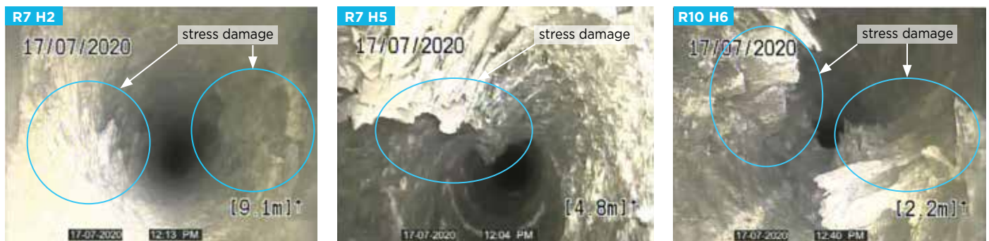
Figure 1. Examples of the varying degrees of deformation observed during the production hole survey
