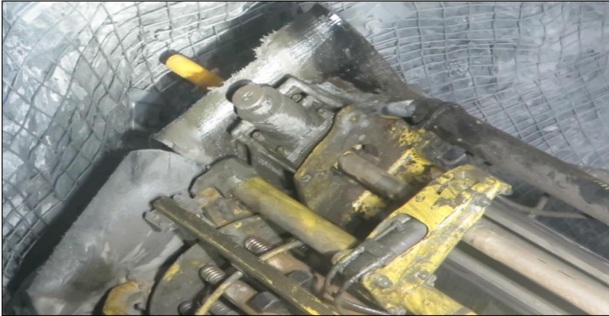
Index drill rod & line up with hole
