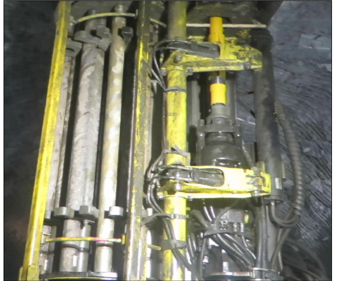
Rotate boom & push LHP through jaws
