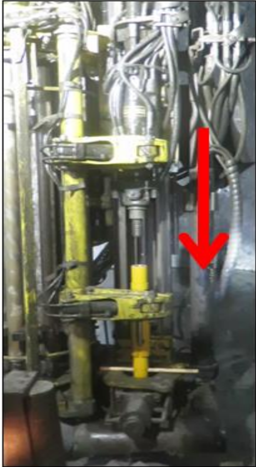
Place in Jaws & locate drifter
